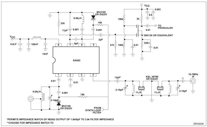
Figure 19. Typical Varactor Tuned Application
