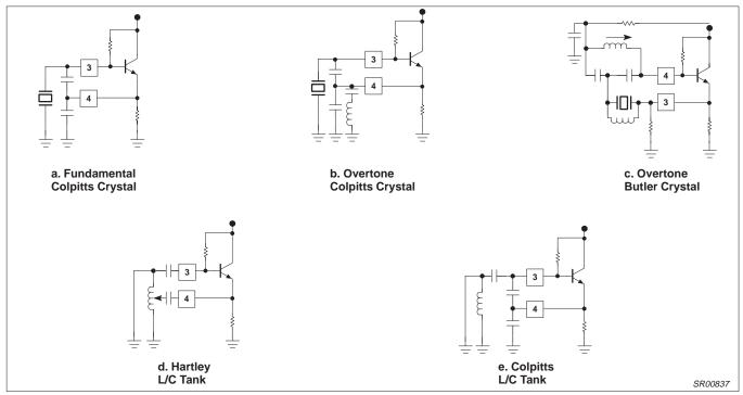
Figure 18. Oscillator Configurations
