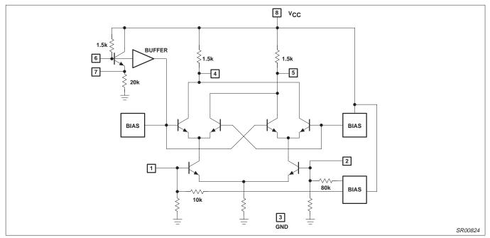
Figure 5. SA602 Equivalent Circuit
