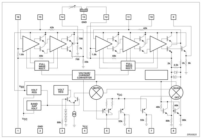
Figure 6. SA604A Equivalent Circuit
