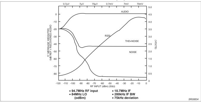
Figure 15. FM Broadcast Receiver (Wide Band)
