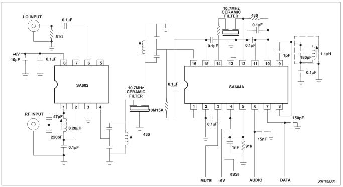
Figure 16. SA602/604A Demonstration Circuit with RF Input of 152.2MHz and IF of 10.7MHz  $\pm$ 7.5kHz
