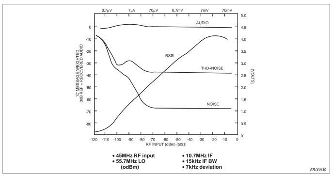
Figure 11. VHF or UHF 2nd Conversion (Narrow Band)
