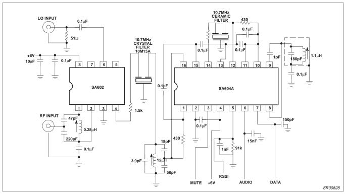
Figure 9. SA602/604A Demonstration Circuit with RF Input of 45MHz and IF of 10.7MHz  $\pm 7.5$ kHz
