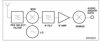
Figure 1. Basic Hetrodyne Receiver
