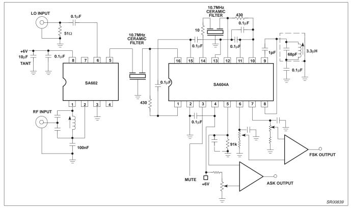
Figure 20. Basic SA602/604A Data Receiver
