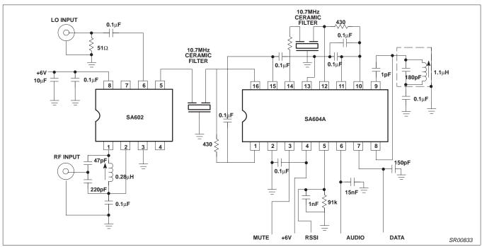
Figure 14. SA602/604A Demonstration Circuit with RF Input of ~100MHz and IF of 10.7MHz ±140kHz
